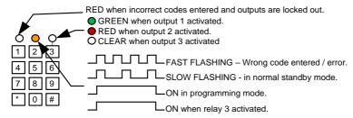
TIP: Flashing amber LED is normal standby mode!
